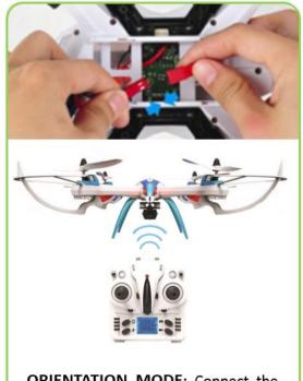
ORIENTATION MODE: Connect the battery to the Tarantula X6. Place the quadcopter on a flat surface and turn ON the Transmitter. LED on the Drone will blink rapidly. When the light remains constant, the process is ready.
