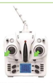
TRIM ADJUSTMENTS: it helps the fine tune the quadcopter flight. Place it on a flat surface and bind it. Switch to 100% speed. Push both, Throttle Stick and Direction Sitck to left-down (as shown in the Picture) for 6 seconds. LED will finishes blinking to complete the adjustment.
